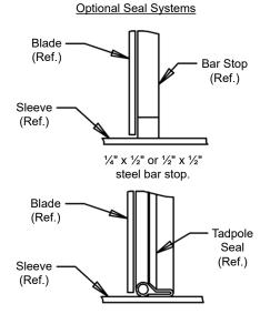
Ept. Fiberglass or Inconel tadpole seal in steel U-clip frame.
